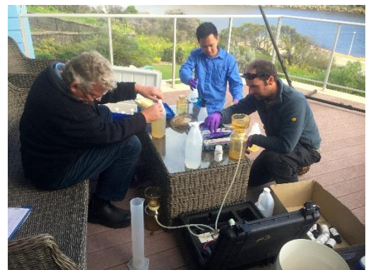
Filtering water samples before being transported to the National Measurement Institute in Perth.
